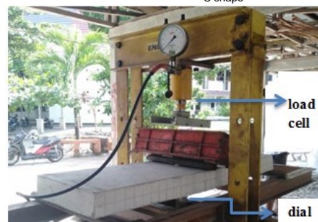
Fig. 4. Detail of slab and Set-up of test
