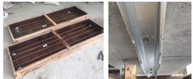
Fig. 3. Normal and Strengthened Slab
